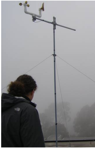
A wind monitoring system, installed on the roof of the Council Civic Offices on Doncaster Hill, is testing the feasibility of wind-generated energy in the Civic Precinct.
